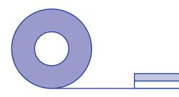
Butyl rubber based self-bonding layer
